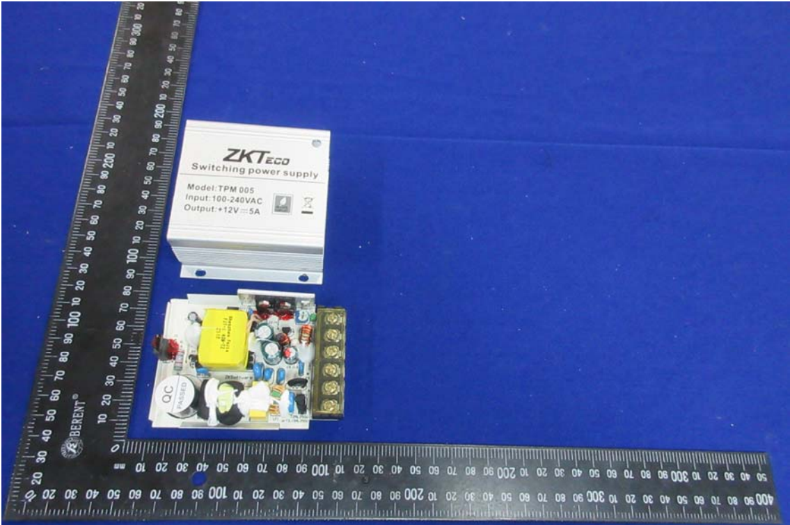
Fig.16 – Power inside view
